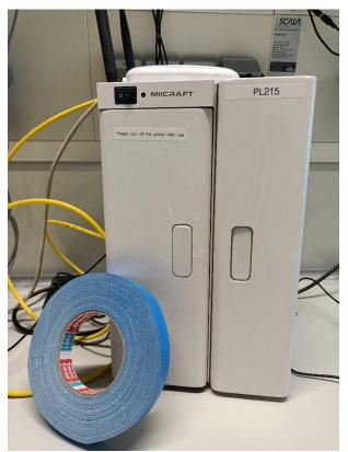
Weight: 8.5 kg Vertical (Z-axis) construction speed 3 cm per hour with 100 micron layers 2 cm per hour with 50 micron layers 1 cm per hour with 30 micron layers
