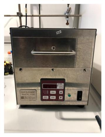
UV+O (atomic oxygen) cleaning method is a photosensitized oxidation process in which the contaminant molecules of photo-resists, resins, human skin oils, cleaning solvent residues, silicone oils, and flux are excited and/or dissociated by the absorption of short-wavelength UV radiation. Atomic oxygen is simultaneously generated when molecular oxygen is dissociated by 184.9nm and ozone by 253.7nm.
