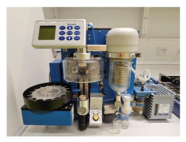
${\sf Biotage}^{\otimes}$  V-10 rapidly dries samples dissolved in both aqueous and organic solvents. It easily evaporates HPLC fractions from purification, high boiling point solvents from synthesis and volatile solvents.
